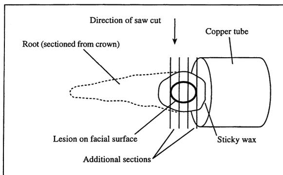
**Fig 5.** Orientation of tooth section in copper tube and direction of saw cuts. Dark circle represents area of suspected lesion.
