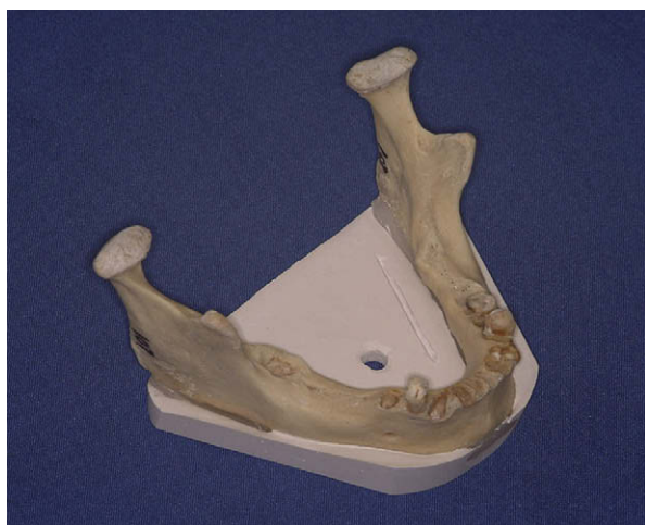
Fig 1. Plaster custom jig for holding dried cadaver mandible.
